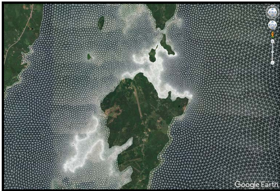
Figure 6. Close-up of Penobscot Bay Model Grid Showing Grid Resolution and Domain Extent at Grindle Point and the Narrows
